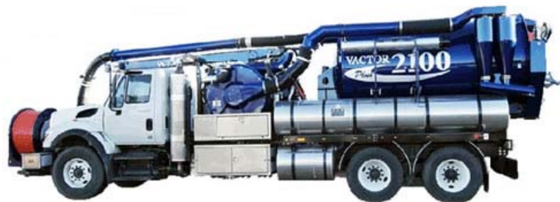
District's Vactor jet cleaning truck
